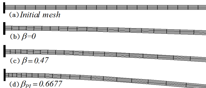
Fig. 4. Deformed shapes and mesh motions during the deformation of under van der Waals force
