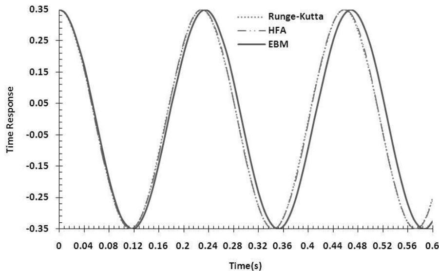
Fig. 2. Comparison between He's frequency amplitude, energy balance method [6] and the fourth-order Runge-Kutta method where  $A=0.35$  and  $V=0$
