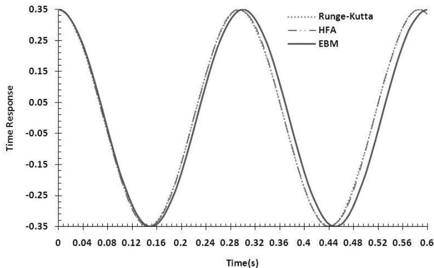
Fig. 3. Comparison between He's frequency amplitude, energy balance method [6] and the fourth-order Runge-Kutta method where  $A=0.35$  and  $V=16$
