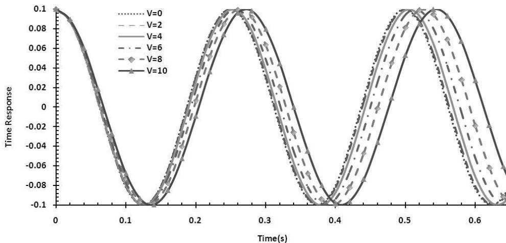
Fig. 6. Microbeam deflection for  $A=0.1$  and different values of non-dimensional electrostatic load
