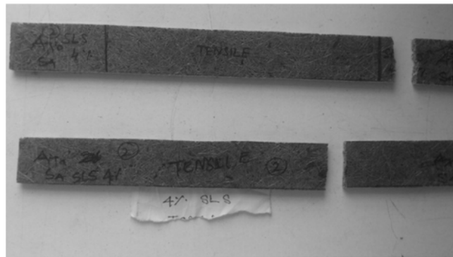
Fig. 8. (a) Specimen for tensile test (4% SLS and 10 mm length), (b) Specimen for tensile test (4% SLS and 20 mm length)
