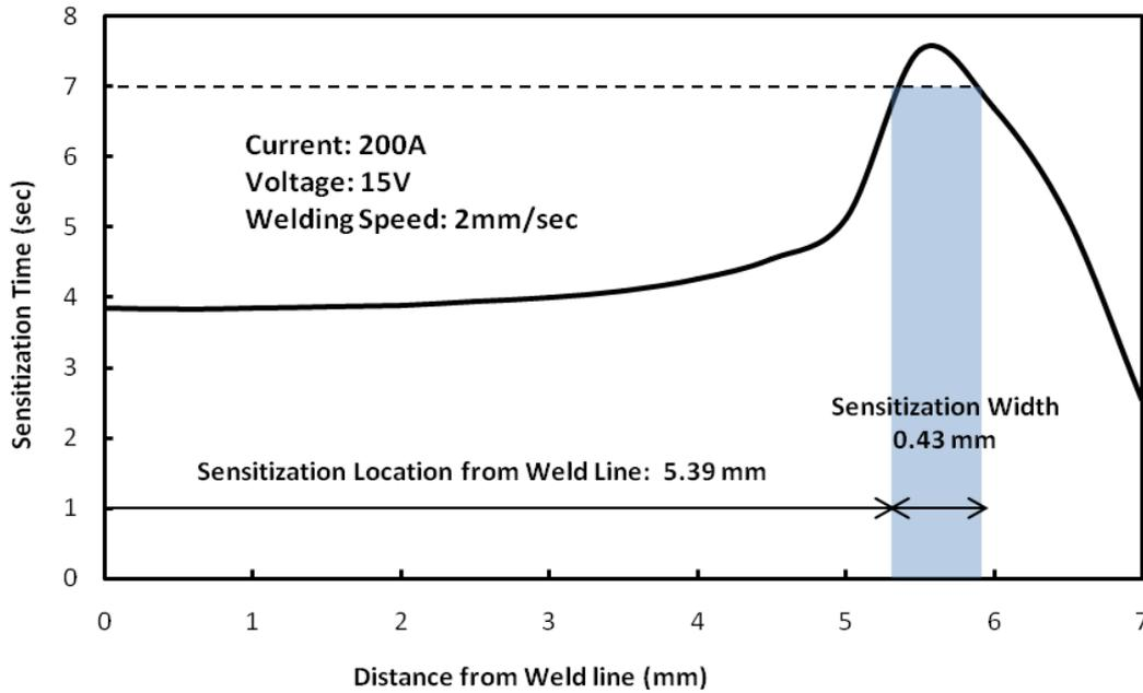
Fig. 4. The exposure time to the temperature range of sensitization as a function of the distance from weld line. For the present conditions, a 0.43 mm wide sensitization zone occurs at the distance of 5.39 mm away from the weld line
