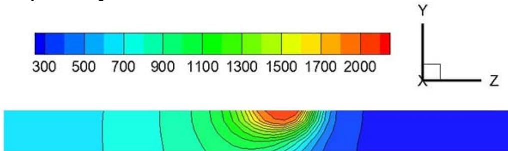
Fig. 2. Temperature distribution at current of 200A during welding in the Y-Z cross section of the welded plate. All temperatures are in Kelvin (K)
