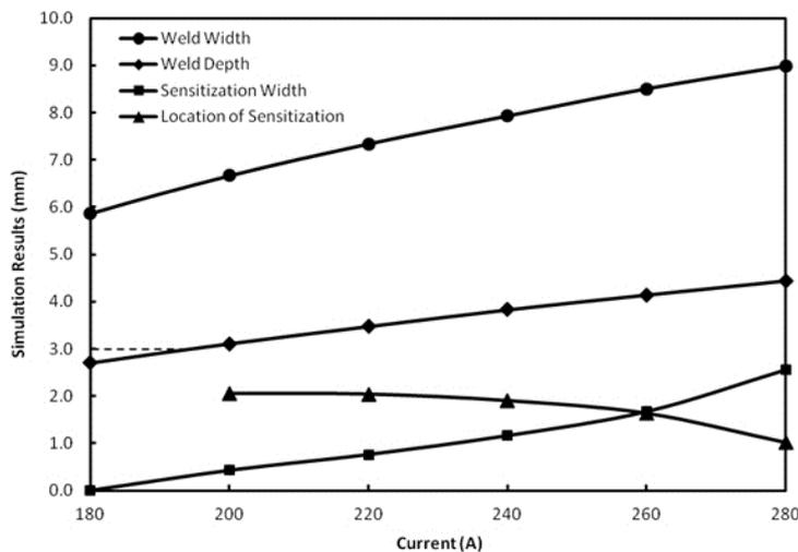
Fig. 5. Weld depth, weld width, sensitized size and its location from weld line as a function of welding current. The size of sensitization increases and the sensitization comes closer to the weld line with the increase in the depth and width of the weld
