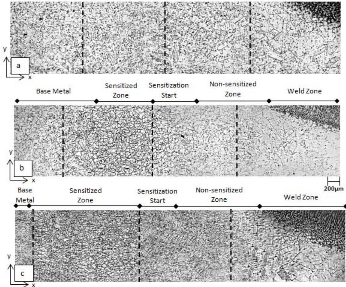
Fig. 9. Microscopic images at different locations from weld line a) sample 1, b) sample 2 and c) sample 3. Each figure consists of four images taken from particular locations away from the weld line.
