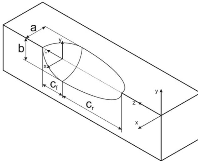
Fig. 1. Schematic model of the Goldak's double-ellipsoid heat source. Two ellipsoidal sources (one in the front quadrant of the heat source and the other in the rear quadrant) are combined
