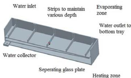
Fig. 2. Sectional 3D view of basin tray
