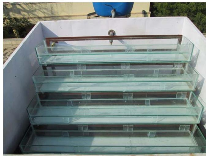
Fig. 3. Photographic view of stepped solar still
