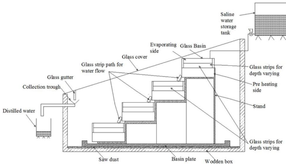
Fig. 1. Schematic diagram of stepped solar still
