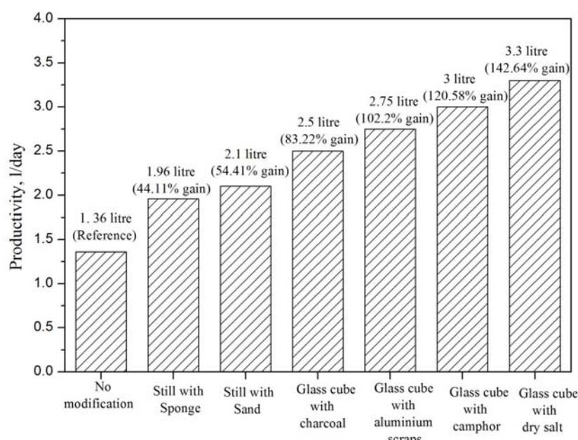
Fig. 9. Comparison of gain percentage of various materials
