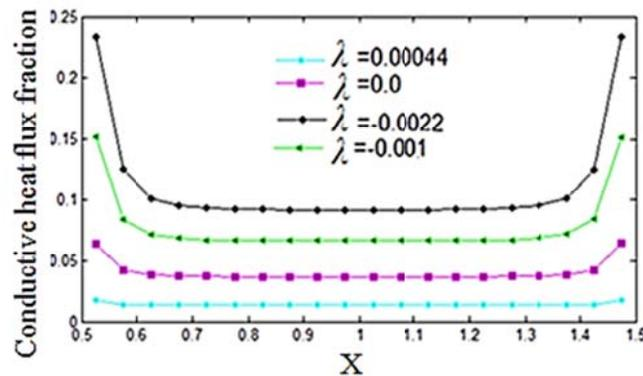
Fig. 10. The effect of conductivity-temperature coefficient on the conductive heat flux fraction over the bottom wall, for ( $N_{cr} = 0.00033, \epsilon_w = 1.0, \beta = 1.0, \omega=0.5$ )
