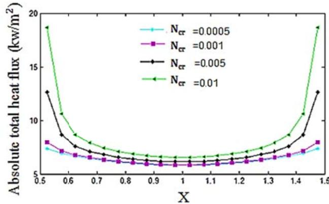
Fig.12. The effect of Conduction-radiation parameter on the absolute total heat flux over the bottom wall, for ( $\lambda = 0.00044, \epsilon_w = 1.0, \beta = 1.0, \omega = 0.5$ )
