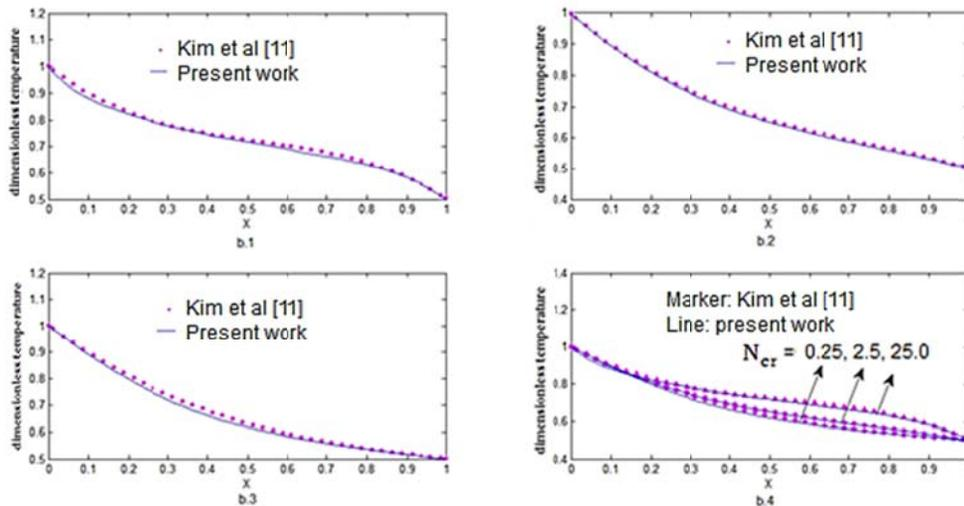
Fig. 3b. Variation of mid-plane temperature ( $Y=0.5$ ) for case 1; (b.1:  $N_{cr}=25.0$ ), (b.2:  $N_{cr}=2.5$ ), (b.3:  $N_{cr}=0.25$ ), (b.4: effect of  $N_{cr}$ ), comparison with the results of Kim et al [11]
