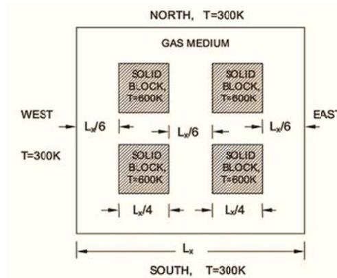
Fig. 4a. Computational domain considered for validation of pure radiation problem (case 2) four similar solid blocks placed symmetrically
