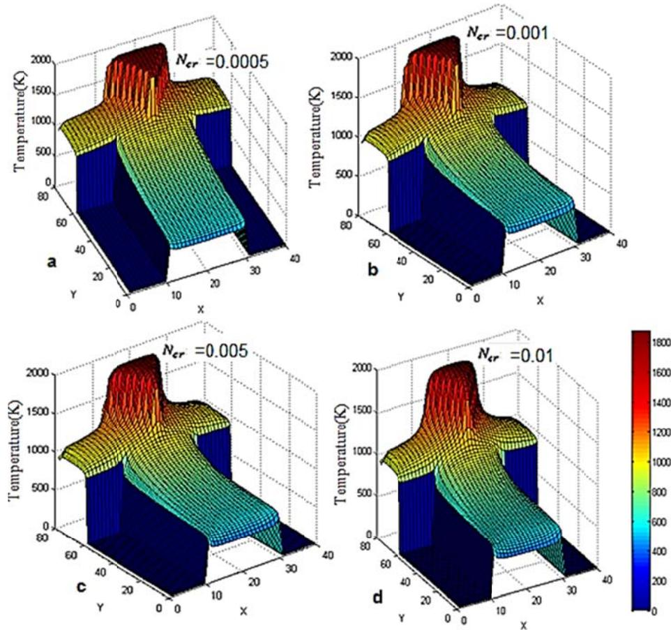
Fig. 13. The effect of Conduction-radiation parameter on the temperature distribution within enclosure.
