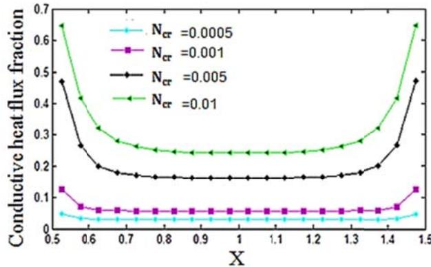
Fig.11. The effect of Conduction-radiation parameter on the conductive heat flux fraction over the bottom wall, for ( $\lambda = 0.00044, \epsilon_w = 1.0, \beta = 1.0, \omega = 0.5$ )
