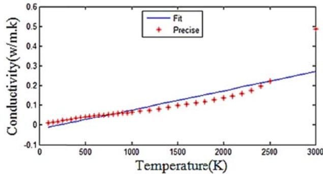
Fig. 6. Variation of thermal conductivity with temperature
