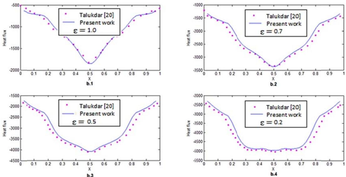
Fig.4-b. Radiative heat flux along the south boundary of the enclosure for different emissivities (b.1:  $\epsilon = 1.0$ ), (b.2:  $\epsilon = 0.7$ ), (b.3:  $\epsilon = 0.5$ ), (b.4:  $\epsilon = 0.2$ ), comparison with the results of Talukdar et al. [20]
