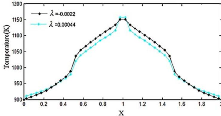
Fig. 8. Temperature distribution in the section AA', for two different values of  $\lambda$ , ( $N_{cr} = 0.00033, \epsilon_w = 1.0, \beta = 1.0, \omega=0.5$ )
