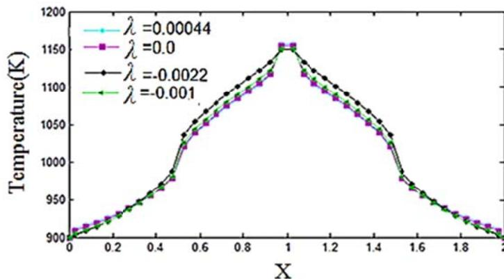
Fig. 7. The effect of conductivity-temperature coefficient on the distribution temperature in the section AA', for ( $N_{cr} = 0.00033, \epsilon_w = 1.0, \beta = 1.0, \omega=0.5$ )
