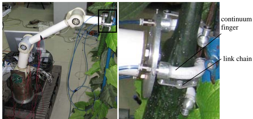
(a) cucumber harvesting robot (b) enlarged end-effector Fig. 14. Three-fingered cucumber harvesting end-effector
