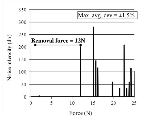
Fig. 5. Bonding strength between the substrate and coating
