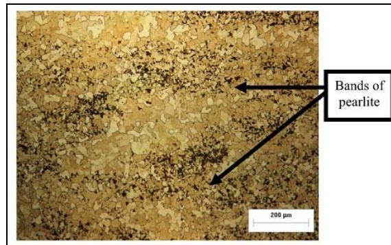
Fig. 7. The pearlite microstructure in the boundary between base metal and HAZ before weld repair
