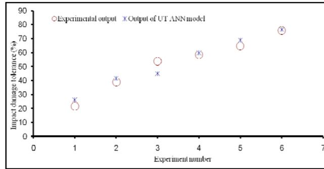
Fig. 19. Experimental and ANN output for validation of ANN model using UT parameters
