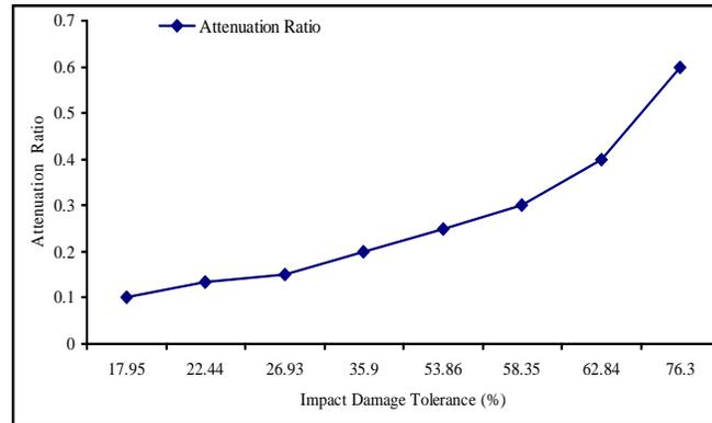
Fig.14. Impact damage tolerance vs attenuation ratio
