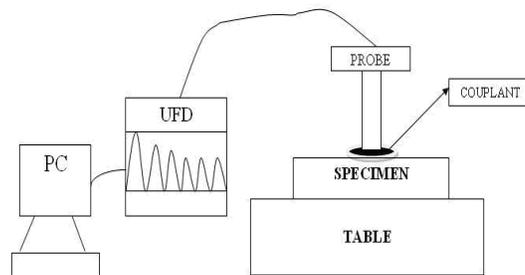
Fig. 2. Schematic experimental diagram for ultrasonic set up
