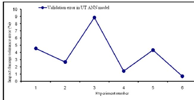
Fig. 18. Validation error of ANN model using UT parameters
