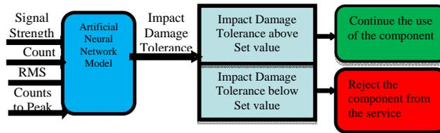
Fig. 17. Decision making algorithm for assessment drop impact damage by online technique
