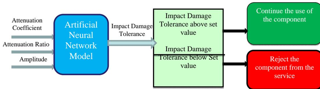
Fig. 20. Decision making algorithm for the assessment of drop impact damage by offline
