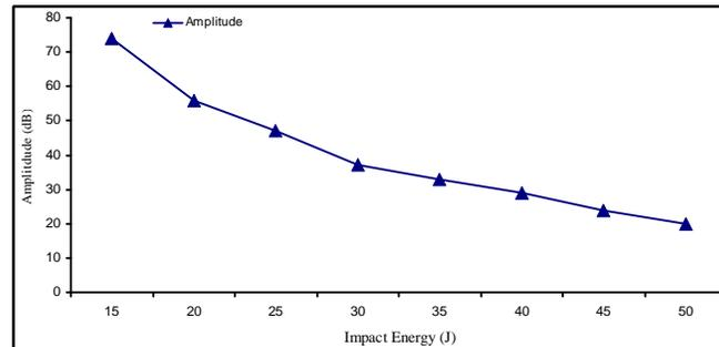
Fig. 9. Impact energy vs amplitude
