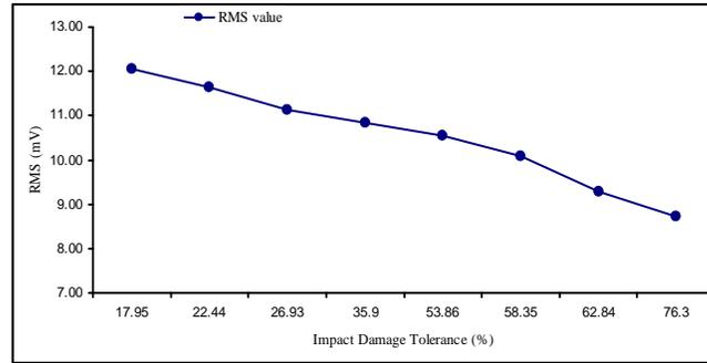
Fig. 8. Impact damage tolerance vs RMS value
