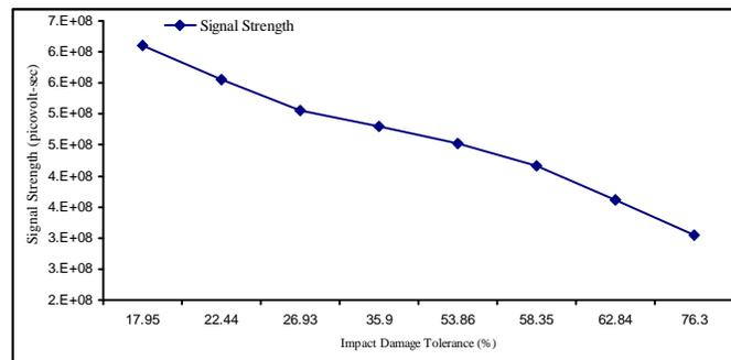
Fig. 6. Impact damage tolerance vs signal strength
