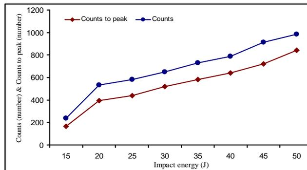
Fig. 3. Impact energy vs counts, counts to peak
