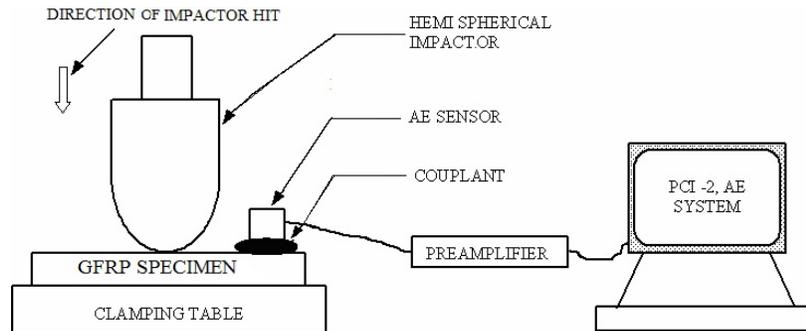
Fig. 1. Schematic experimental diagram for acoustic emission set up
