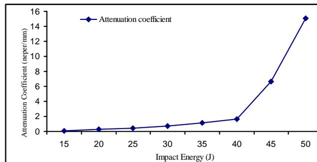
Fig. 10. Impact energy vs. attenuation coefficient
