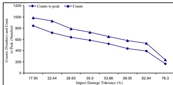
Fig. 7. Impact damage tolerance vs counts, counts to peak
