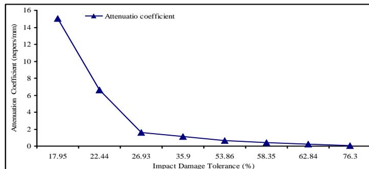
Fig. 13. Impact damage tolerance vs attenuation coefficient
