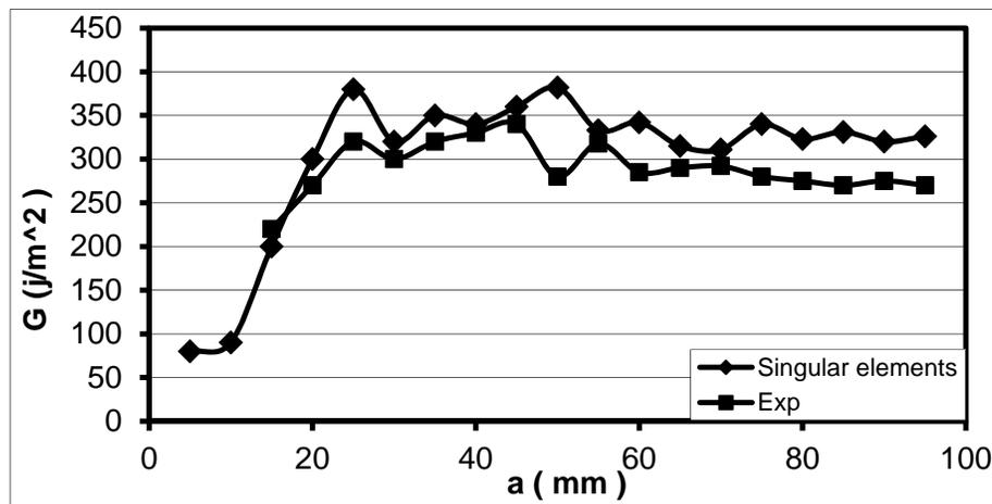
Fig. 14. Curves of strain energy release rate relative crack length for singular elements
