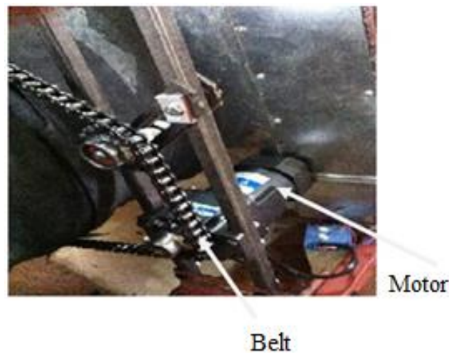
Fig. 3. Illustration of the driving mechanism of the DW
