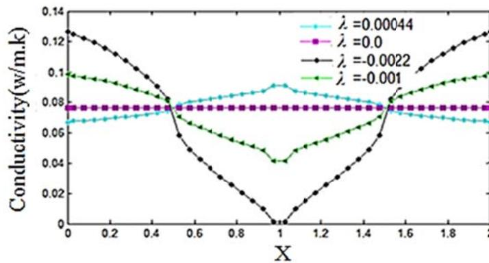
Fig. 9. Variation of thermal conductivity in the section AA'
