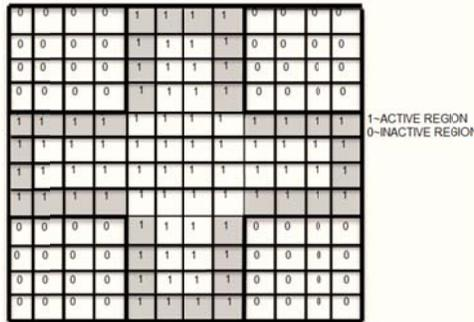
Fig. 2. A domain with blocked-off/inactive region
