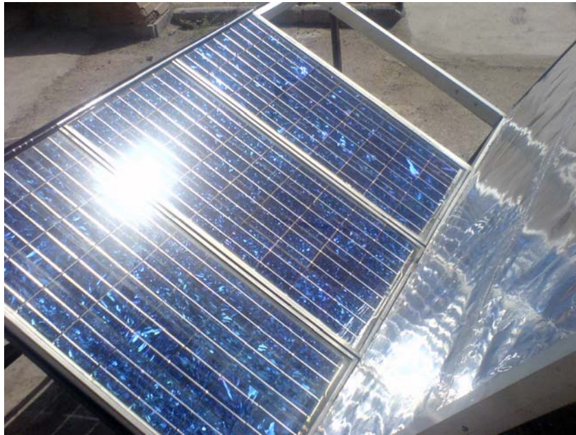
Fig. 1. The experimental setup consists of PV modules equipped with Aluminum foil booster reflector
