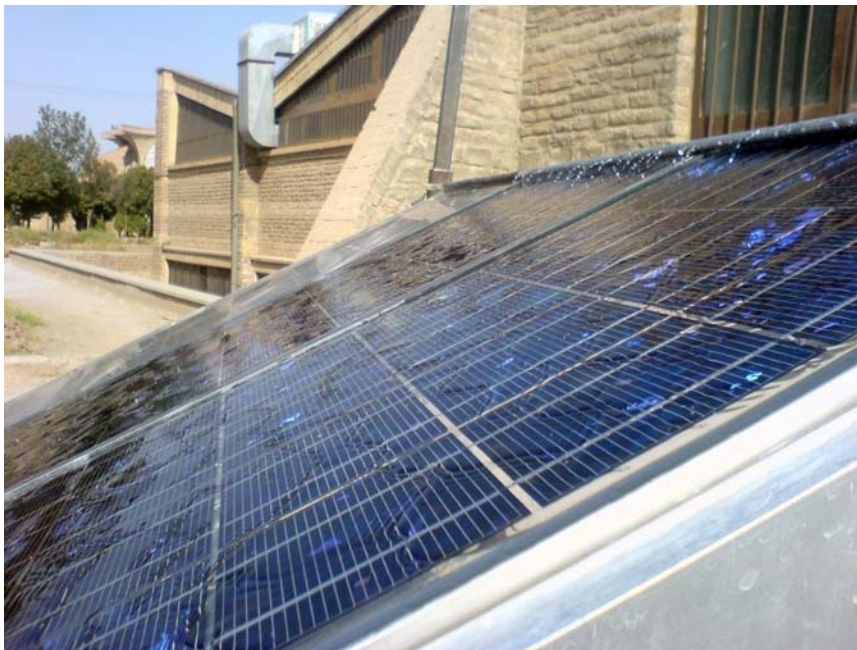
Fig. 2. Transmitting water from the pump over the cells front
