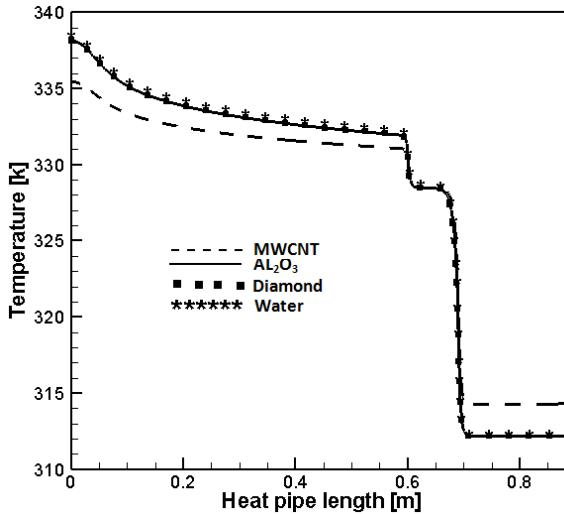
Fig. 4. Heat pipe temperature distribution;  $q=1180 \text{ W}$
