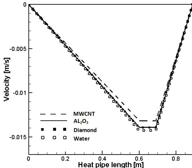
Fig. 6. The effect of different nanoparticle materials on the liquid velocity at  $q=1180\text{ W}$
