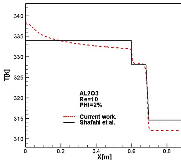
Fig. 3. Comparison of heat pipe temperature distribution with analytical results given by Shafahi [3] at  $Re=10$
