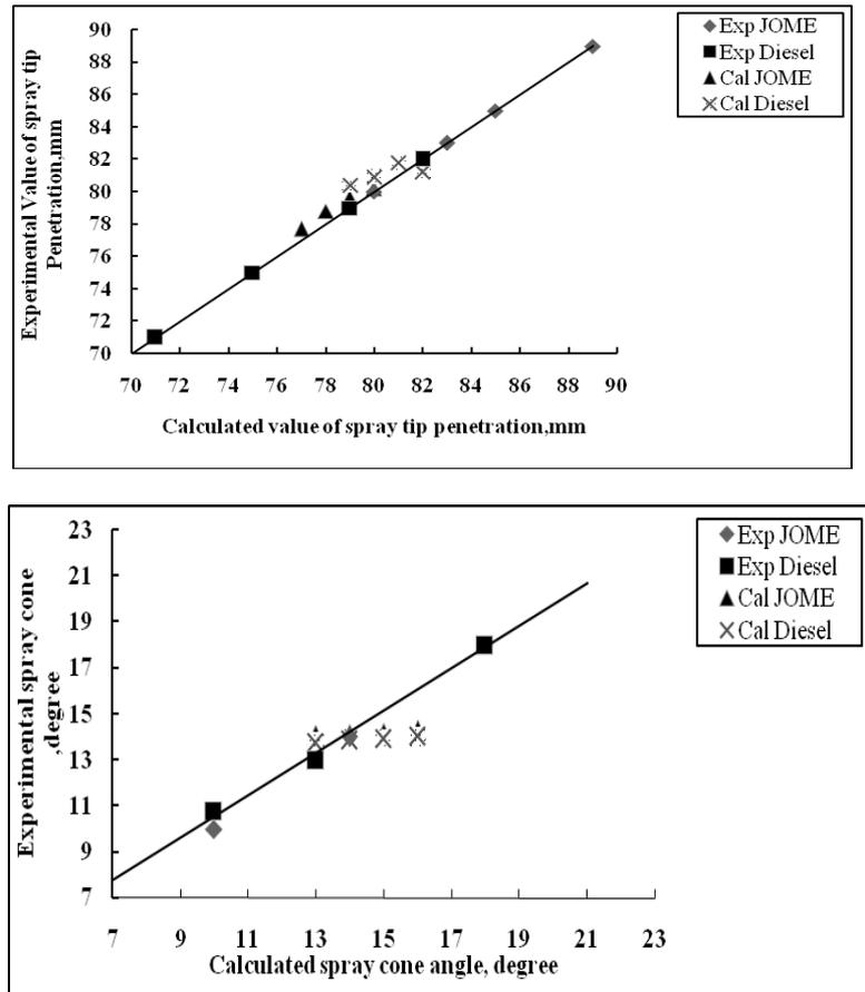
Fig. 9. Comparison between calculated and measured spray cone angle and spray tip penetration
