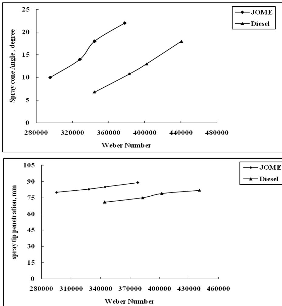
Fig. 6. Spray cone angle and spray tip penetration versus Weber number for various injection pressures (180,200,210 and 230 bar)
