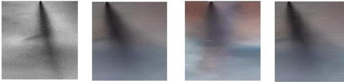
Fig. 4. Images of biodiesel spray development (injection pressure 180,200,210 and 230 bar), ambient pressure 1bar and ambient temperature 300 K)
