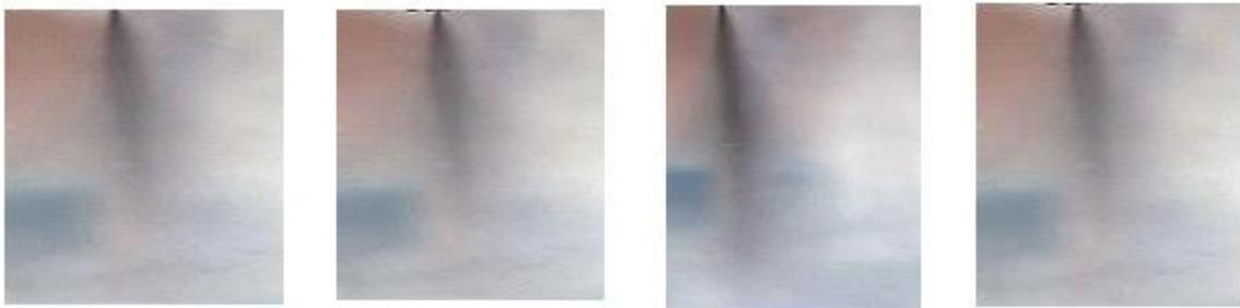
Fig. 3. Images of diesel spray development (injection pressure 180,200,210 and 230 bar), ambient pressure 1bar and ambient temperature 300 K)
