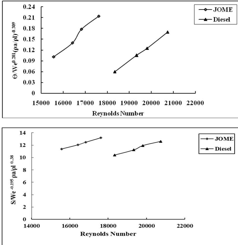
Fig. 8. Effect of dimensionless numbers on spray cone angle and spray tip penetration
