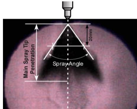
Fig. 1. Definition of spray tip penetration and spray cone angle
