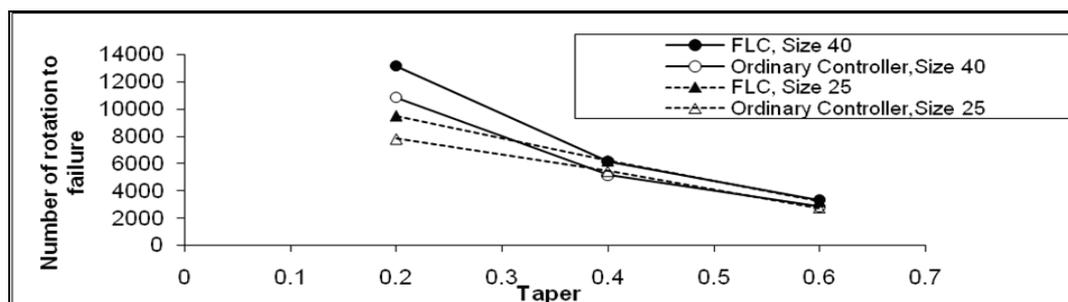
Fig. 9. Mean values for file rotation to failure in a fuzzy control system VS ordinary control system in size 25 and 40 in different tapers
