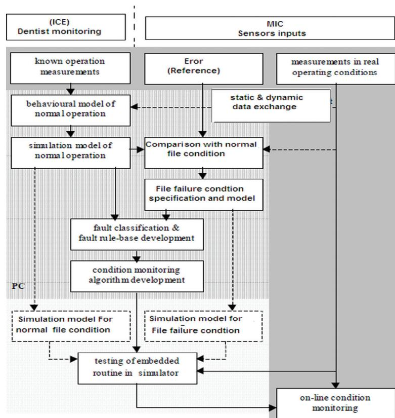
Fig. 5. Simulation algorithm method
