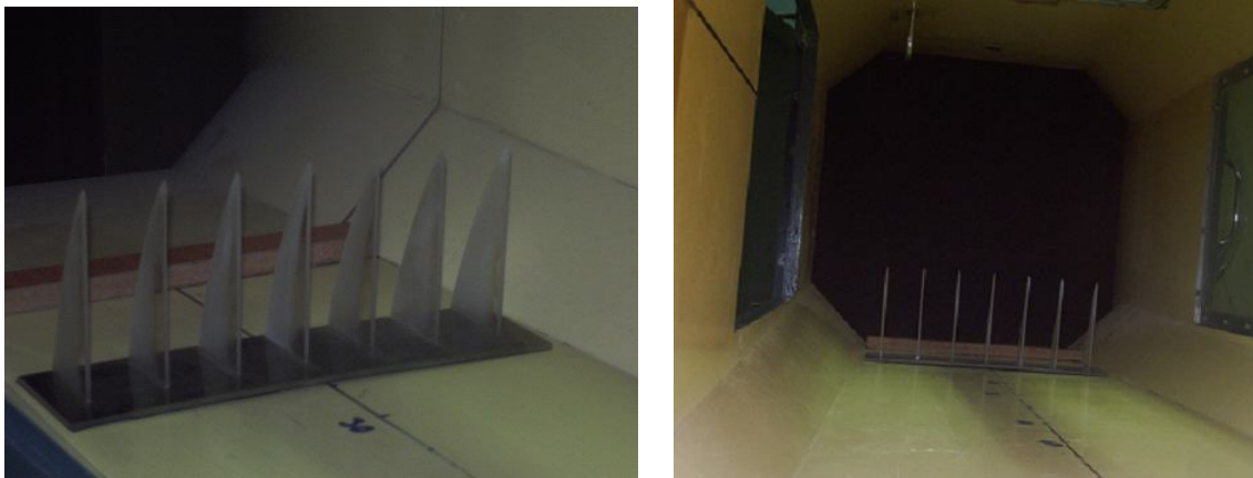
Fig. 1. Barrier and elliptic wedges at the inlet of the wind tunnel for thick boundary layer generation
